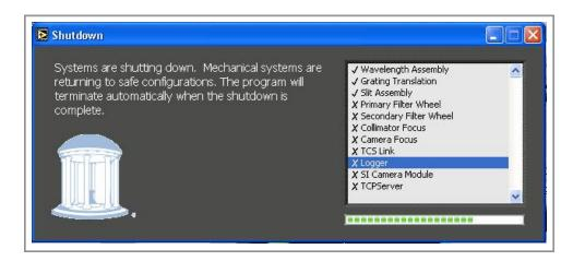
The X's will change to checkmarks as each subsystem is stored. Please wait for all systems to shutdown before proceeding. Once this occurs, the *Shutdown* window will disappear, and the GSCS *Labview* program will stop running. The operators may now shut power off to the spectrograph without harming any motors.
